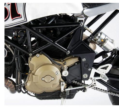
dedicated ECU ignition, and STM Evo slipper clutch," d'Acunto recounts. "This dramatically changes the curve and the power—104 horsepower at peak—giving to the bike a racing spirit with real explosion after 4000 rpm."
